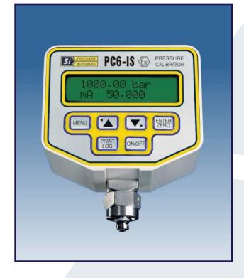
The PC6-IS is the Intrinsically Safe version of our popular PC6 Pressure Calibrator specifically designed for use in Hazardous Environments such as those found in the off-shore and petrochemical industries.
